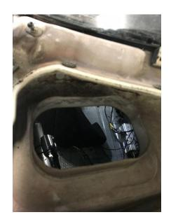
6) Once the screen is removed or repositioned you will be able to fit the cabin filter in the hole with a snug fit, the metal brim around the hole is very thin and can be massaged to fit the cabin filter securely in the hole.
