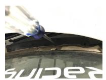
5) Once the cover is removed you will see the hole where the cabin filter goes. It is covered by a metal screen which will either need to be removed (recommended) or pushed down to allow the filter to sit on top. If you decide to remove it you will need to cut out the 4 spots where the mesh is spot welded to the cowl, there will be 2 welds on the front and 2 on the back of the opening.
