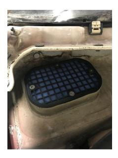
7) Once the filter is installed, reinstall using the steps above in reverse.
